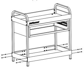
7. Attach one Handle (6) to each end, using eight Bolts (9), Washers (16), and Lock Nuts (14).
