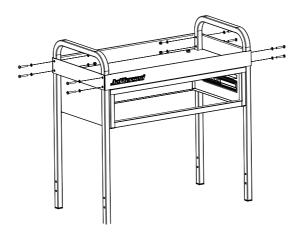
5. Lock Locking Swivel Casters.6. Attach one Post (3) to each corner of Drawer/Shelf assembly and Lower Shelf, using twenty four Bolts (10), Washers (16) and Lock Nuts (14) total, eight on
