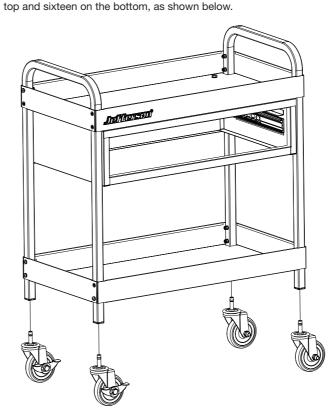
4. Attach Upper Shelf (2) to Drawer Frame (1), using four Bolts (12), eight Washers (15), and four Lock Nuts (13).
