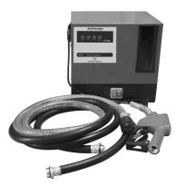
This is a 230V mobile pump which is perfect for dispensing diesel or light fuel oils such as paraffin from drums or tanks. The equipment comprises of an electric motor, vane oil pump, flow meter and fuel nozzle. This dispenser has been designed for a wide variety of noncommercial uses and is ideal for refuelling vehicles and equipment in garages, construction sites or agricultural environments. The pump kit is reliable, easy to operate and maintain.
