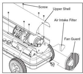
Figure 10. Air Intake Filter Acess
