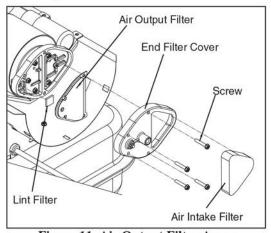
Figure 11. Air Output Filter Acess
