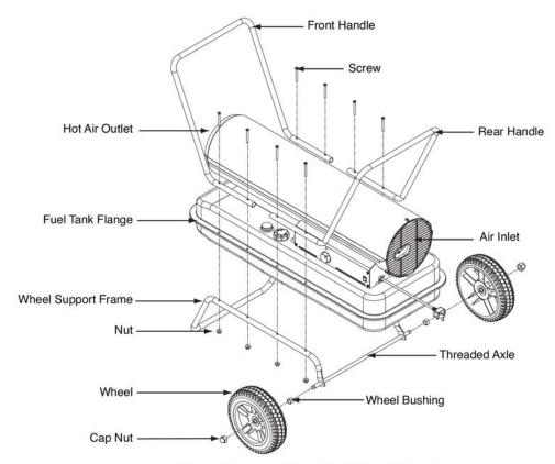
Figure 7. Assembling Handel and Wheels
