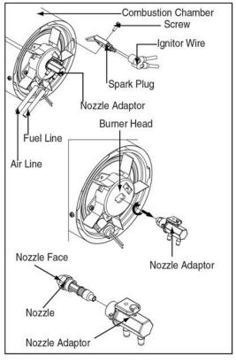
Figure 13. Remove Dirt in Nozzle
