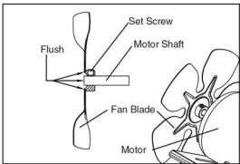
Figure 12. Fan Assembly
