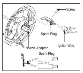
Figure 14. Clean & Regap Spark Plug
