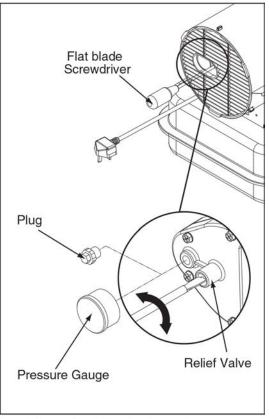
Figure 17. Adjusting Pump Pressure
