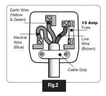
• Ensure that the power supply matches voltage requirements specified on the equipment and that the plug is wired correctly and fitted with the correct fuse (See Fig.2).
