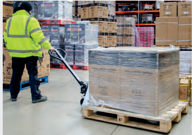
PUMP CONTROL HANDLE ALLOWS 3 FUNCTIONS: LOWER, NEUTRAL, LIFT
